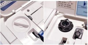
There are two types of foot pressure – adjustable and Non-adjustable
