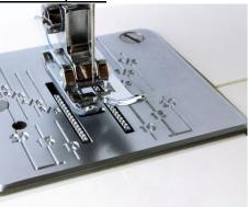
This is metal plate covers your bobbin and fits over the feed dog. Most sewing machines have engraved lines with seam width guides.
