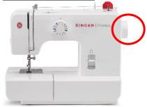
Often found on the side of the machine (red circle), you turn the dial clockwise or anti-clockwise for your needle to go up or down.
