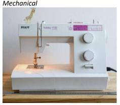
These sewing machines are controlled by using dials. You have several dials performing different functions – adjusting stitch width and length, dial for stitch choice, dial to move your needle up and down. You are in control.
