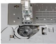
These are much easier to load. You just drop the bobbin into the machine and follow the instruction/images for the thread and voila, it is done. They are also easy to clean.
