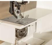
As per the image above, they are found at the front of the machine. They can be fidgety to load, trying to fit a bobbin at the odd angle with your fingers holding onto the bobbin. Then making sure it has slotted in correctly is time consuming. Front loaders are known to jam more often.
